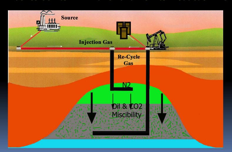
**Gas Flooding EOR** -- also known as *miscible* gas flooding -- is one of the leading enhanced oil recovery (EOR) technologies employed for recovering the stranded, trapped oil, left behind in pressure-depleted oil reservoirs after initial primary oil recovery has ended.
